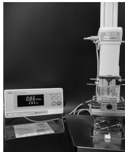
Fig 2: Tuning-fork Vibration Viscometer SV-A (2ml sample measurement is possible)
