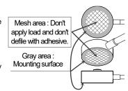
Peel and shave adhesive using cutter and etc. when removing the load cell.
