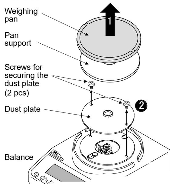
3. Confirm that the "UPPER SIDE" label is visible (up). Using the two screws supplied, install the breeze break lower plate on the balance.
