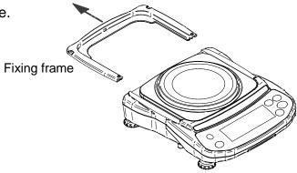
2. Attach the breeze break to the breeze break frame.
